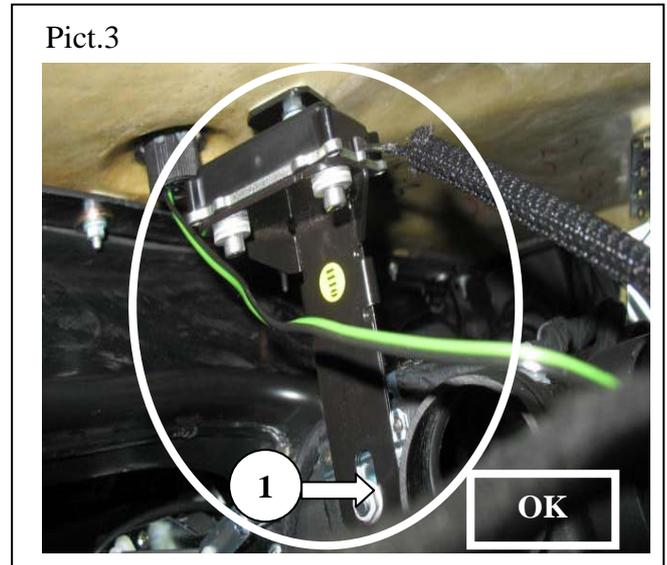
1.5 If the SDARS antenna is in the wrong position (Pict.2), unscrew the bolt (1-Pict.3) and remove the bracket with SDARS antenna (1-Pict.4).
